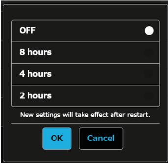
Restarts after the time selected on the menu has elapsed when no operation is performed.
