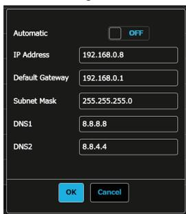
The settings are shown below when connecting to the Web page of the receiver immediately after purchase or after initialization by pressing the reset button of the receiver.
