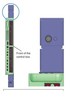
Approx. tightening torque: 4.5 N·m ± 0.1 N·m
