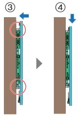
Confirm that the upper and lower hooks are properly hooked on the mount fittings. 3 Slide the cabinet module so the stoppers on the rear butt against the wall mounts.
