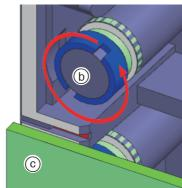
Restore the LED module to its original position after aligning.
