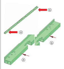
Fit so the gaps between the screw heads and fittings are approx. 5 to 7 mm.
