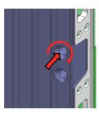
Use the LED module height adjustment tool (DPVF4987ZA/X1) (page 51) or a commercially available hexagonal tool (Hex No.3) to turn the screw **clockwise** to make the magnets higher and align the surfaces of the LED modules.
