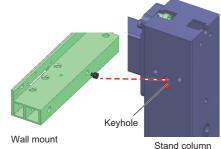
Take care with the work, supporting the wall mount with your hand so that it doesn't fall. 3 Secure the supplied M6-50 screws to 6 places on the stand (upper section).
