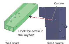
Take care with the work, supporting the wall mount with your hand so that it doesn't fall. 5 Secure the supplied M6-50 screws to 6 places on the stand (lower section).
