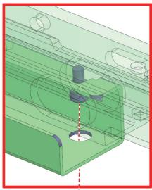
This temporarily fixes the cable covers, so now secure completely through the hole underneath.
