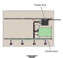
Installing on the wall mounts
