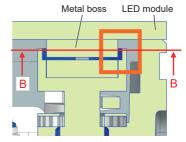
The design specifications allow for 0.5 mm of movement in the X and Y directions for the LED module in the cabinet.
