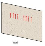
3 Put the wall mount back up against the wall and secure using M8 screws that are appropriate for the type of wall construction (8 places).
