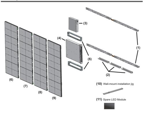
The components are used when the Control Box is attached to the rear of this unit.
