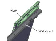
There are stoppers attached to the left side of the cabinet, so when hooking the cabinet aim to put the center of the cabinet slightly inside the edges of the wall mounts.
