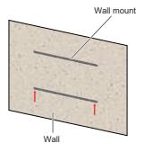
7 Fit the cable covers in 3 places on the lower wall mount.
