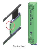
Refer to the numbers on the colored tags adhered to the cables, and match them to the numbers on the control box when connecting. Insert fully so that the tab locks into place.
