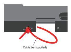
3 Take the AC cable bundle that has been bundled by the cable spiral tube, and use the hook and loop fastener (supplied) to hang it from the cable tie.
