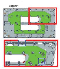
The metal bosses on the LED module fit into these 2 position determining magnets, and thereby regulate the position in the X and Y directions.
