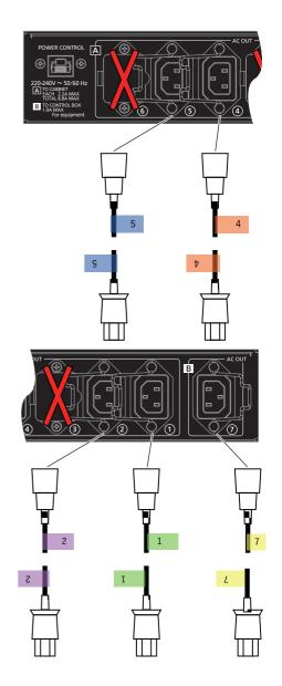
The AC OUT terminals on the power box are of the C14 type. After fully inserting the AC cords, attach the cable retaining clips on the power box side.
