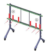
(a) On the stand side, the locations with fixing blocks and the columns at the side
