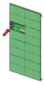
Restore the LED module to its original position after aligning.
