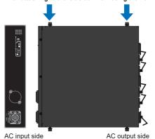
Loosen so that there is a gap of approx. 3 to 5 mm between the screw heads and the box. Keep to a maximum of 6 mm so that they do not fall out at some stage.
