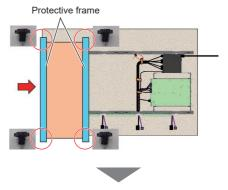
Remove the protective cushion from the surface of the cabinet module.
