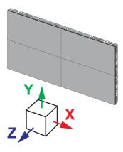
4 LED modules are attached to each individual cabinet in the Z direction using magnets.
