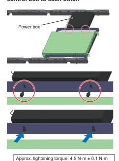
8 Tighten the screws that were left loose
