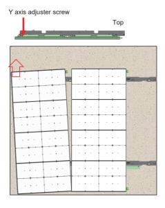
Slide the left cabinet to the right so the stoppers butt against the wall mounts. Next slide the right cabinet to the left to close the gap.
