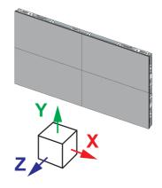
4 LED modules are attached to each individual cabinet in the Z direction using magnets.
