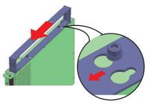
(3) Tighten the screws (2 places on each side for a total of 4 places)
