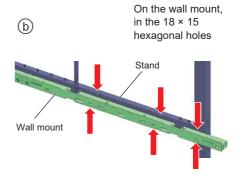
6 Secure the cable covers (3 places) to the wall mount with the screws (M6-12) included with the cable covers.
