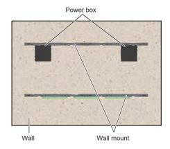
1 Screw the included M6-12 screws into what will be made the top side of the power box.
