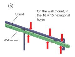
Approx. tightening torque: 4.5 N·m ± 0.1 N·m
