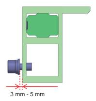
7 Slide the cable covers over the screws you fitted, fitting the cuttings onto the screws.
