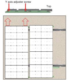
Slide the left cabinet to the right so the stoppers butt against the wall mounts. Next slide the right cabinet to the left to close the gap.
