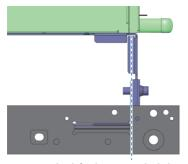
Look for the rectangular hole in the wall mount as a guide for where to place the anchor bracket.
