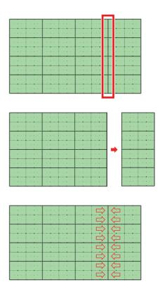
If the problem is not solved by joining without gaps between the cabinets, slide the LED modules that are neighboring the gaps and make it so the gaps are equal with the surrounding LED modules.
