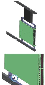
Approx. tightening torque: 4.5 N·m ± 0.1 N·m
