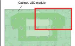
Each individual LED module is secured by magnetic force in the Z direction using 15 magnets.
