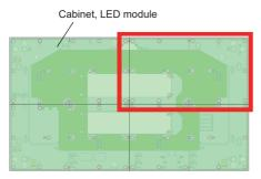
Each individual LED module is secured by magnetic force in the Z direction using 15 magnets.
