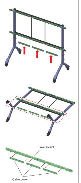
Fit so the gaps between the screw heads and wall mount are approx. 3 to 5 mm.
