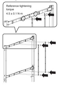
5 Check that the trestle bases, the vertical poles and the cross bars are accurately put together with no backlash.
