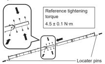
Turn each bolt approximately five turns. Do not fully tighten these bolts.
