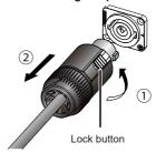
Turn the connector counterclockwise (1), pulling the lock button on the plug towards you, then pull it out (2).
