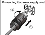
Plug the connector fully into an outlet (1) and turn it until you hear a click (2).
