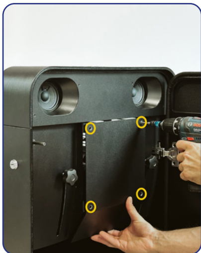
2. Unscrew the projector cable cover (HEX3)
